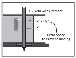
Figure 107. Adjusting the fence with an <sup>1</sup>/<sub>64</sub>" offset.
